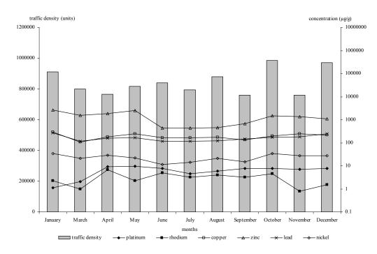
Figure 4: Monthly average concentration of Pt, Rh, Cu, Zn, Pb and Ni of East Tunnel with monthly traffic density for year 2006
