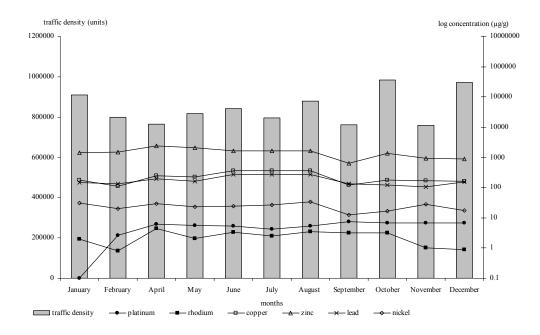
Figure 2: Monthly average concentration of Pt, Rh, Cu, Zn, Pb and Ni of West Tunnel with monthly traffic density for year 2006
