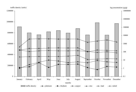
Figure 3: Monthly average concentration of Pt, Rh, Cu, Zn, Pb and Ni of Escape Tunnel with monthly traffic density for year 2006
